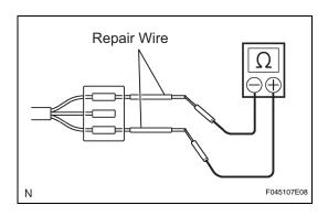
(b) Use a repair wire to check the connector if it is impossible to check the resistance from the rear of the connector.
